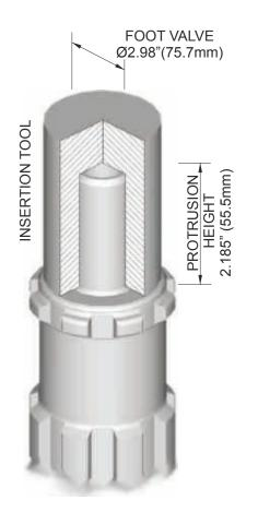
The Hyper 121 Hammer is designed to accept button bits with a N120 footvalve.
