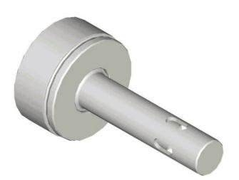
5. Assemble the two Control Tube Buffers and the 'O' Ring around the Control Tube, then push the assembly into the Tube Holder. Coat the outside of the assembly with rock drill oil and insert it into the Backhead end of the Wearsleeve
