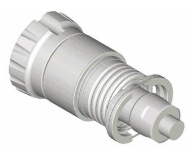
4. Assemble the Chuck, Chuck Release Washer and Bit Retainers around the Bit ensuring the Chuck and Bit Retainers are fitted with new 'O' Rings... Cover the threads with a Copper based grease. Then screw the Chuck fully in until there is no gap between the Wearsleeve and the Chuck Release Washer.
