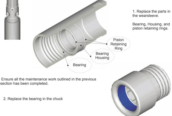
3. Lay the Wearsleeve on two wooden blocks, support the chuck end so as to raise the sleeve 50mm - 70mm off the ground this will make it easier to screw in the chuck assembly.
