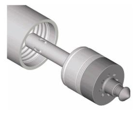
3. The Valve Chest along with the Check Valve arrangement can now be pulled from the Backhead end. The reamaining control tube buffers etc, will also come out at this stage. Should these parts be stuck, lifting the wearsleeve at the chuck end slowly, should allow the piston to fall onto the back parts and allow these parts to move and allow them to be removed.
