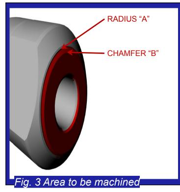
During the working life of the hammer the Striking Face on the Piston may become dented or deformed (see *fig.2*). To prevent this face from cracking, or chipping, the Piston should be returned to a lathe where the strking face can be re-machined flat and then have the outer radius and inner chamfer reformed (see *fig.3*)...
